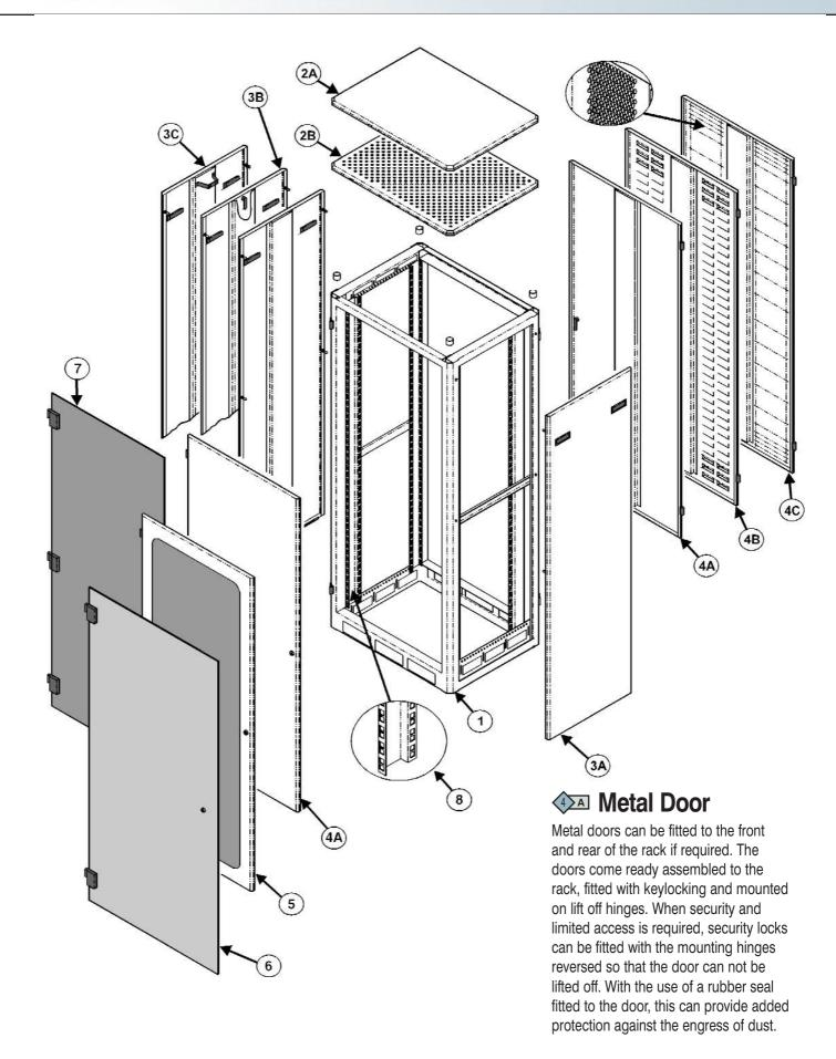
Material: 1.0mm Zinc Coated Steel Finish: Powdercoat Ripple
